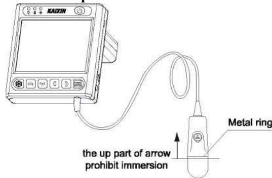
Fig. Probe regular disinfection
